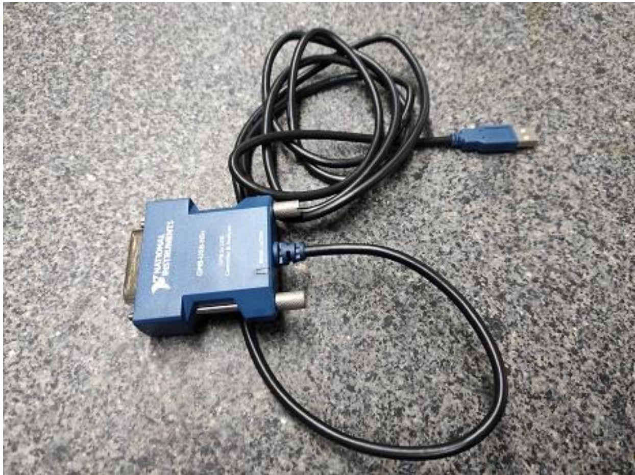
Figura 6. Interfaz GPIB-USB-HS de National Instruments.
